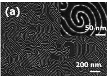
various types of patterns with long-range order. The researchers suggest that varying processing parameters, including deposition time, metal ion concentration, and molecular weight of the block copolymer, could produce nanowires of different properties suitable for a variety of applications.
